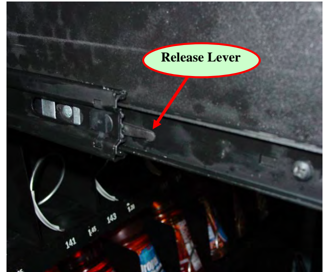
Figure 20: Location of Bottle Shelf Release Lever
