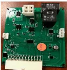
**Cabinet Control Environmental Board** – controls the Refrigeration Unit & Condenser Fan, Evaporator Fan, LED Lighting, Encapsulated Temp Sensor, and 24VDC & 5VDC power distribution.
