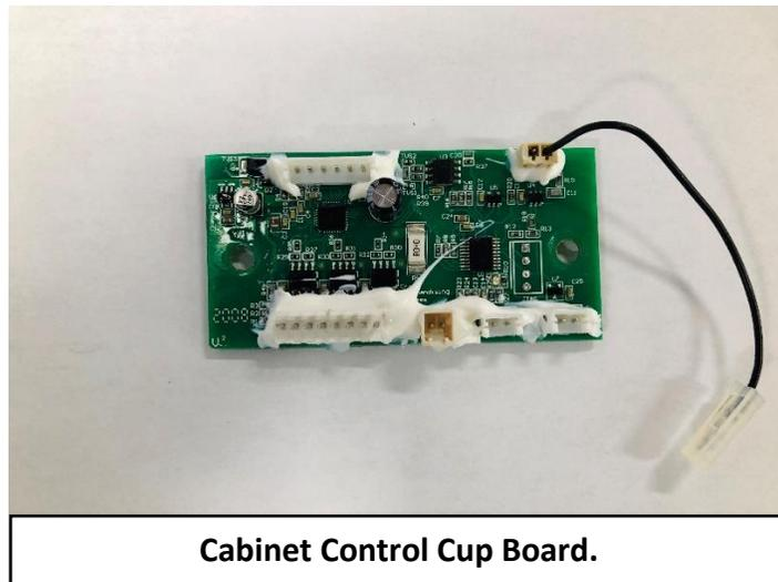
4. Picker still will not cycle, with the left Motor Power Interrupt Door Switch activated and the Picker at home position inside the Cup, go to Cup Test and ensure the VMC D5 Picker Home Switch Diagnostic Red Light is On, and that the VMC D7 Picker Out Switch Diagnostic Green Light is Off.
