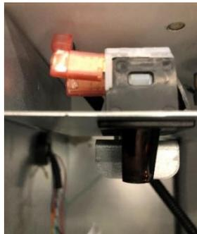
**View of Left (Motor Power Interrupt) Door Switch.**
