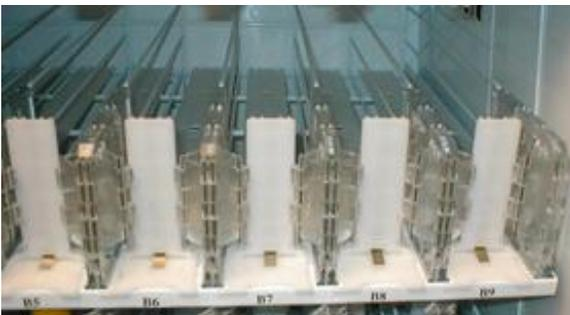
Typically, there are 5 Shelf assemblies in every Vender; however, this can vary depending upon the configuration specified at the time of ordering. Each can/bottle Shelf consists of 9 or 7 columns. Each Shelf is capable of holding a variety of packages. The Shelf assembly consists of the Tray, where all of the following parts are mounted: Double Gate assembly and the Slide/Pusher assembly. These items are discussed in detail below.
