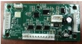
**Cabinet Control X Motor Board** – controls X Motor movement and sense the X Home Switch Signal.
