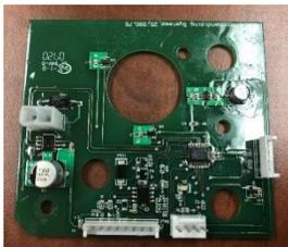
**Cabinet Control Port Board** – controls the Port Vend Sensor, Port Open & Close Sensors, & the Port Motor.
