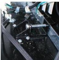
The Refrigeration Deck Clamp assembly is located on the left side of the Cabinet base plate. Its purpose is to secure the Refrigeration assembly tight against the vertical base plate for refrigerated air flow in to the Cabinet. A 7/16" wrench or socket is needed to adjust the bolt. The Refrigeration Unit also has a locating pin on the bottom of the Refrigeration Unit base plate to ensure alignment for Refrigeration gasket seal to the vertical base plate.
