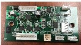
**Cabinet Control Cup Board** – controls the Delivery Cup Sensor, Picker/Plunger Home & Out Switches, and the Cup Motor. The Y Home Switch plugs into the Cup Motor Board and sends the switch signal on to the Cabinet Control Y Motor Board.
