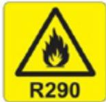
**DANGER:** Propane gas (R290) is flammable, odorless gas. While working on a machine, no smoking and no open flames should be permitted.
