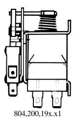
The sequence relay is located on a bracket adjacent to the Vend Relay (credit relay) on the main door and secured with two (2) screws.
