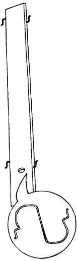
Rear Spacer Assembly 497,073,90x.x3 - Wide 600E 498,071,30x.x3 - Wide 501E 497,073,70x.x3 - Narrow 600E 498,071,40x.x3 - Narrow 501E/276E
