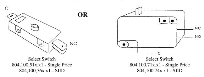
The Select Switch is located in the Select Panel behind the press button and is secured with two (2) screws.
