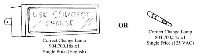
The Correct Change Lamp is mounted in the Coin Insert Casting.
