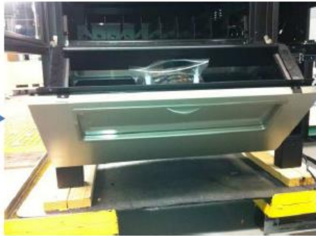
Bin pulled out to access bolts
